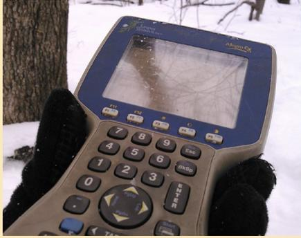
Photo 1: Portable Data Recorder used to record field data measurements (Photo by Sjana Schanning, NRS FIA)
